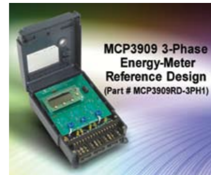
Figure 3: The MCP3909 Energy-Measurement IC Used in a 3-phase Meter, with the PIC18F2520 Microcontroller to Calculate Power.
